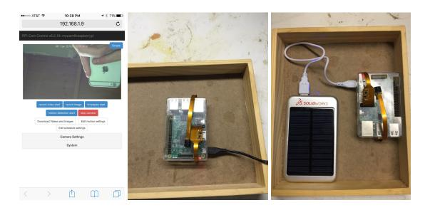
The tethered version of this is less prone to powering down and can be very discrete. I choose the spy camera because it is less than 8mm (.3in) across and comes with a sticky back that can be posted anywhere.
